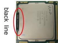
Step 3-2. Locate Pin1 and the two orientation key notches.
