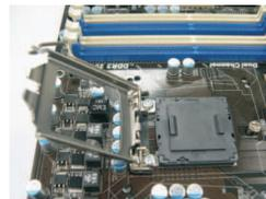
Step 2. Remove the PnP Cap (Pick and Place Cap).
